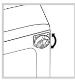
2. If the floor is not perfectly level, compensate for any unevenness by tightening or loosening the adjustable front feet (see figure); the angle of inclination, measured in relation to the worktop, must not exceed 2°.
